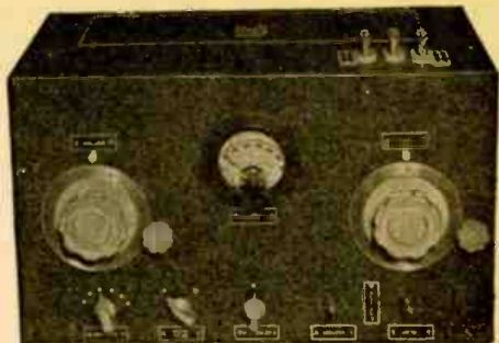
The Comparator. Connection to components being tested are made by posts at upper right.
