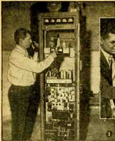
Photo 1—The 250-watt 118.55 Mc. Motorola transmitter. Lt. Ben Denby, at left of rack is using handset for monitoring during adjustment.
